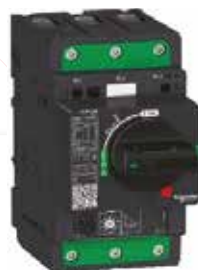
Motor circuit breaker, TeSys GV3 ,4P, 50A, Icu 50KA, thermal magnetic, Everlink terminals
